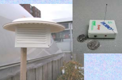
Temperature data logger and housing design – stands 3 to 5 feet above ground
