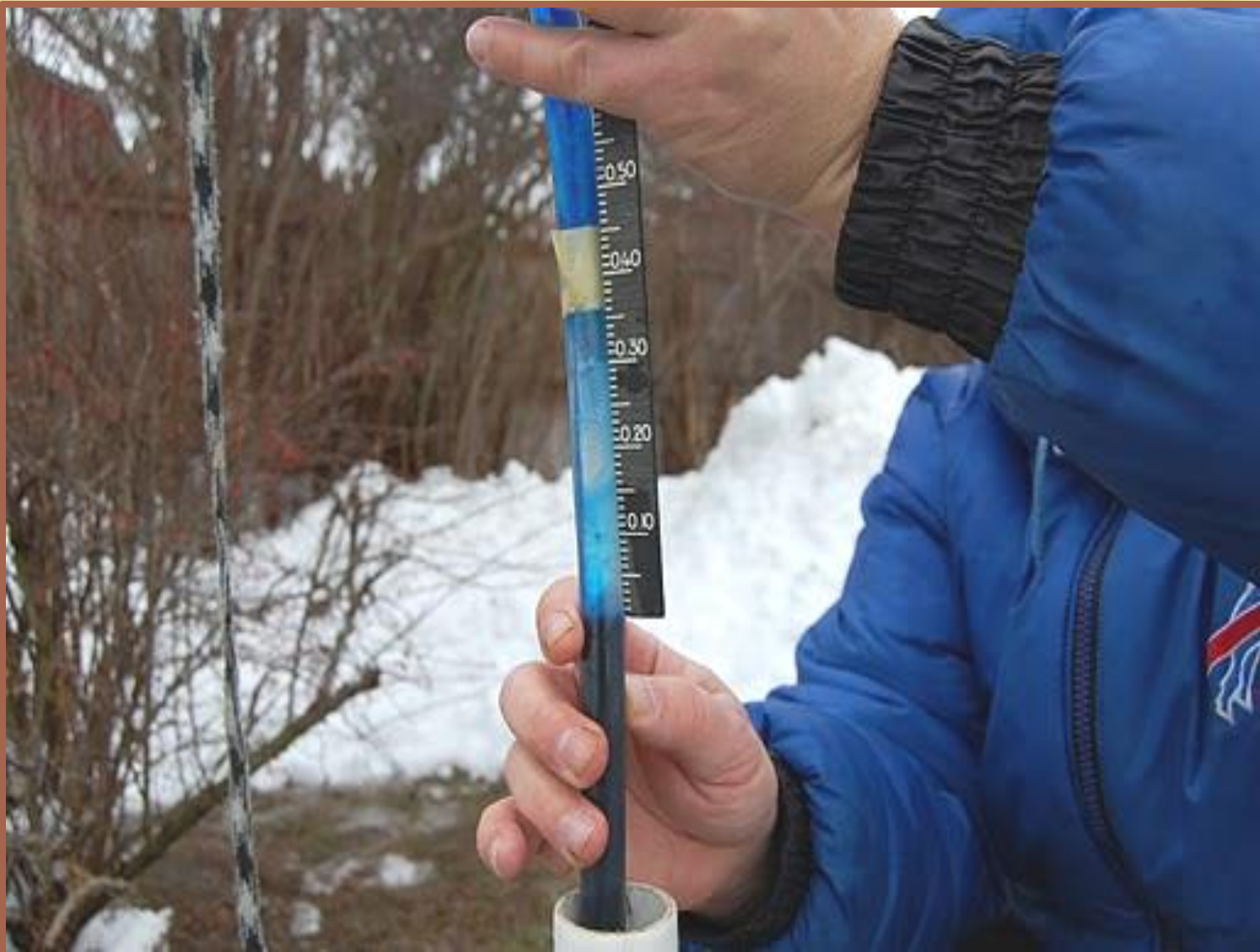
Frost tube measurement showing a frost depth of 8.8 cm (3.5 inches)
