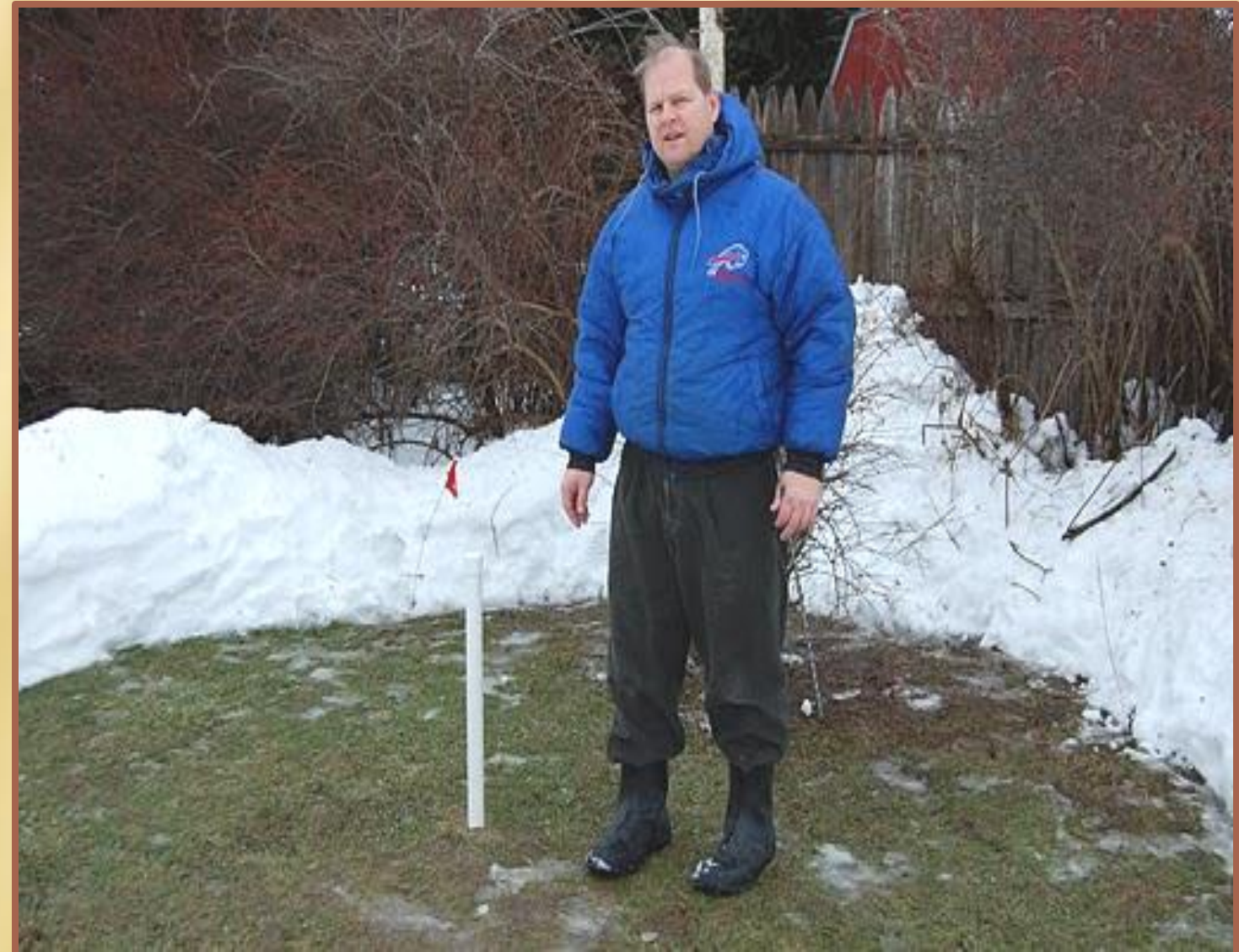
A frost tube (with outer PVC casing) in a snow cleared area.
