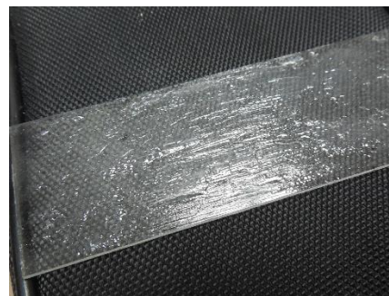
We tested the petroleum jelly down to -23^{\circ}\text{C} and it did not freeze.
