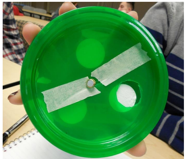
Filter Concept #1: using barometric readings a stepper servo rotates the opening to expose filters at specified altitudes.
